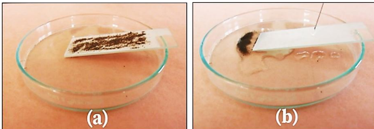
Figure 2. (a) The optical photographs of the soil particles spread on the P3 sample, (b) soil particles washed away easily by the rolling water droplets.
